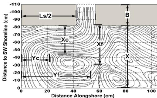
Figure 1 – Dimensional parameters  $X_c$ ,  $Y_c$ ,  $X_f$ ,  $Y_f$  based on laboratory experiments (streamline plot of current field)
